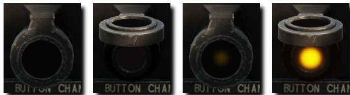
Figure 116: From left to right: Bomb bay doors closed; cover closed; cover open; bomb bay doors open.
