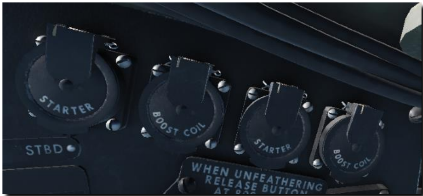
Figure 38: Engine starter buttons.
