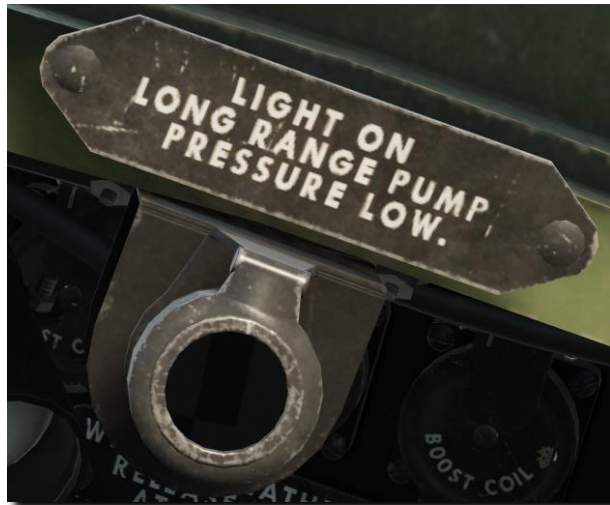
Figure 60: External tank pump pressure low light.
