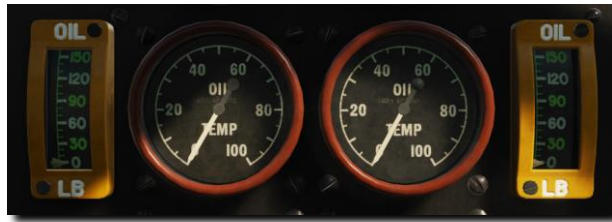
Figure 55: Oil Temperature and Pressure Indicators.
