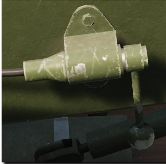
Figure 81: Pilot harness release.
