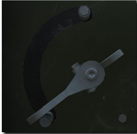
Figure 103: Fuel tank pressurization valve.
