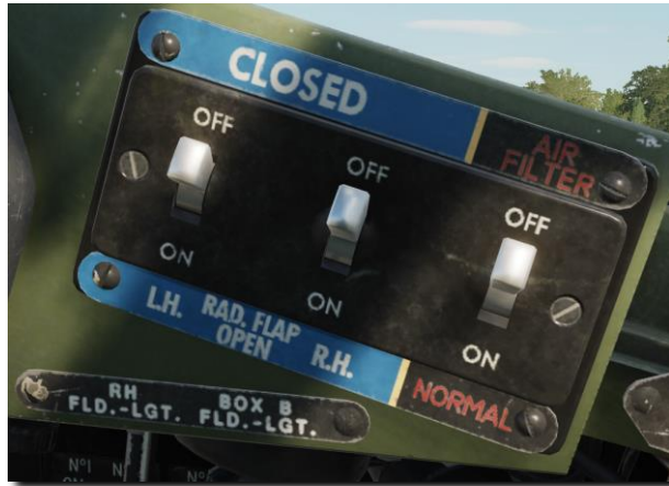
Figure 59: Radiator and air filter switches.
