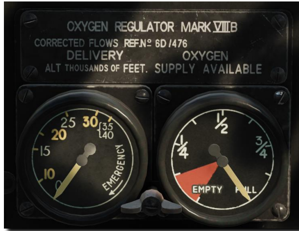
Figure 64: Oxygen indicators Mk. VIII B.
