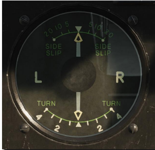
Figure 46: Roll and slip indicator.
