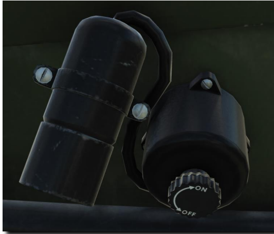
Figure 94: Right cabin flood light.
