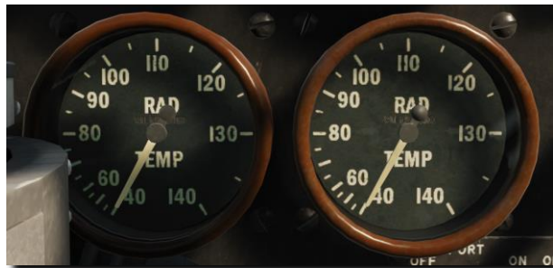
Figure 56: Coolant temperature indicators Mk. VIII.
