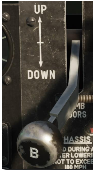
Figure 115: Bomb bay doors open - lever in lower position.
