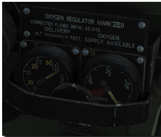
Figure 85: Co-Pilot oxygen regulator.
