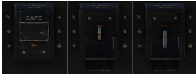
Figure 110: Open the safety cover, depress the switch.
