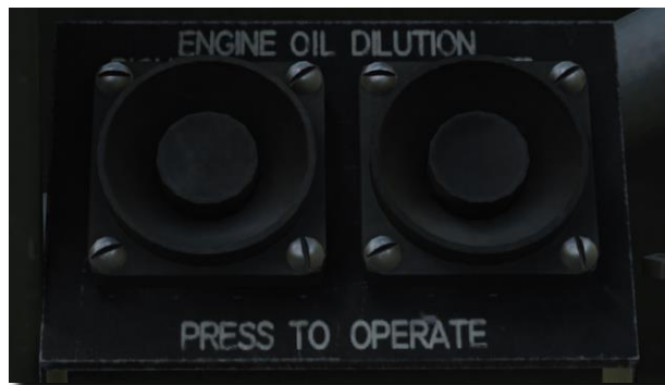
Figure 102: Engine oil dilution buttons.
