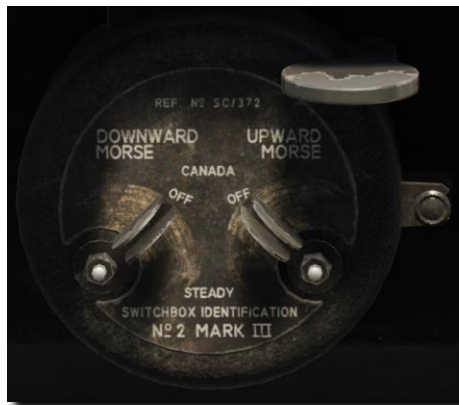
Figure 91: Identification switchbox and Morse key.
