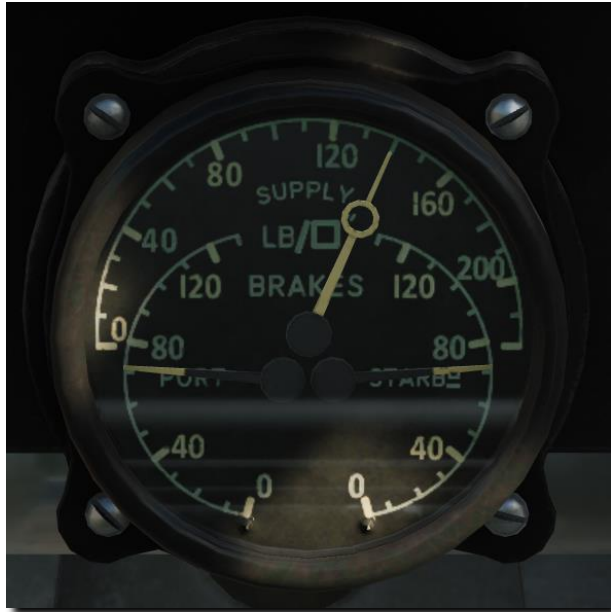
Figure 50: Pneumatic gauge Mk. IC.
