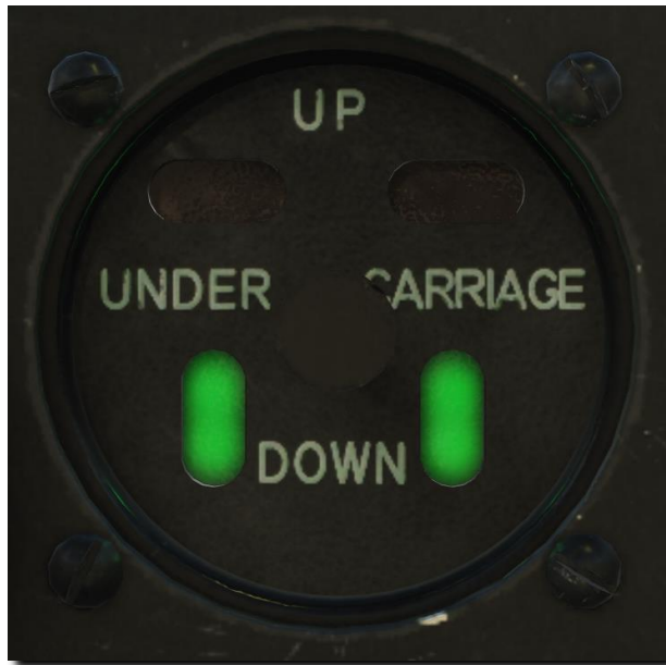
Figure 48: Landing gear indicator.
