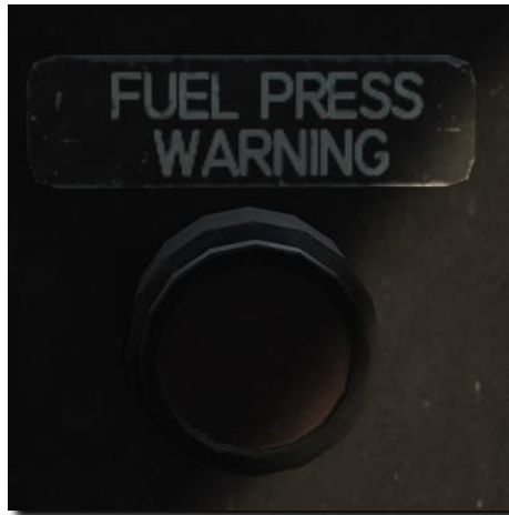
Figure 53: Low fuel pressure lamp.
