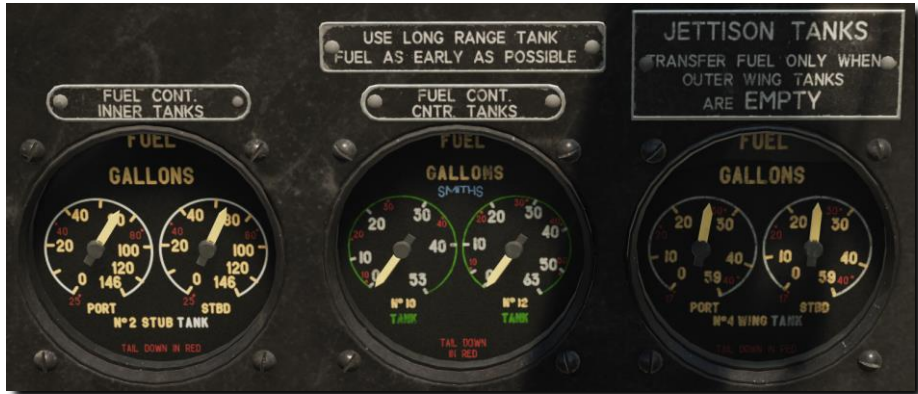
Figure 86: Fuel tanks gauges.
