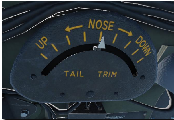
Figure 76: Elevator trim tab indicator.
