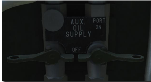
Figure 101: Auxiliary oil supply levers.
