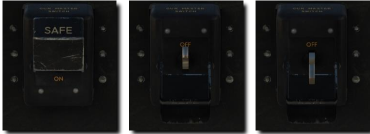
Figure 113: Open the safety cover, depress the switch.
