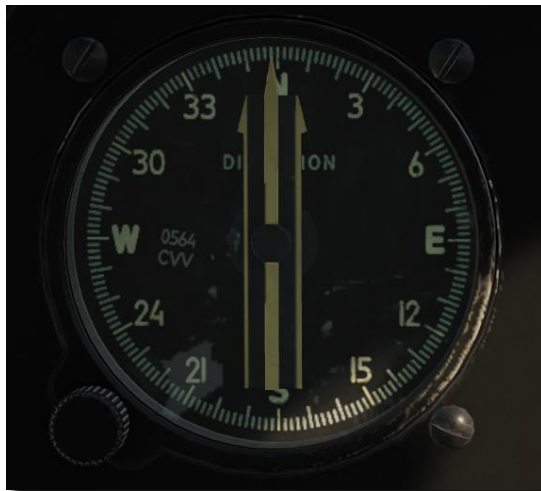
Figure 39: R.I. Compass Repeater.
