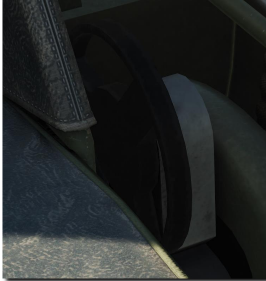
Figure 75: Elevator trimmer wheel.
