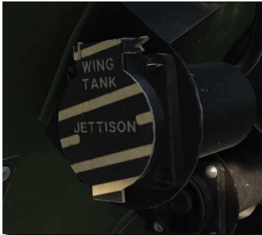
Figure 80: Wing tank jettison.
