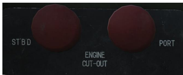
Figure 99: Engine cut-out buttons.
