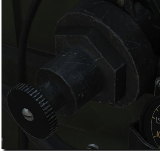
Figure 84: Oxygen high pressure valve.
