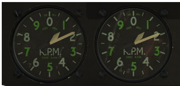
Figure 51: Tachometer Mk. IX G.
