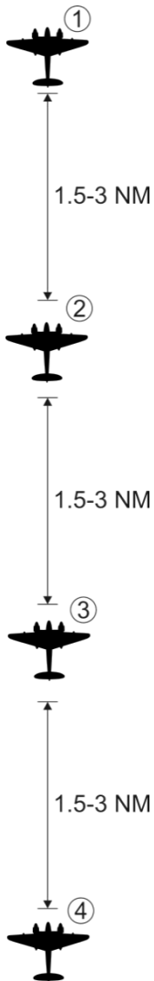
Figure 118: F2. Go Trail. Spacing may be modified by flight lead within a 5,000 foot to 2 NM range.
