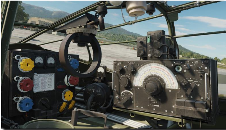
Figure 105: Radio equipment: T.1154 on the left, R.1155 on the right, swivel antenna in the center.
