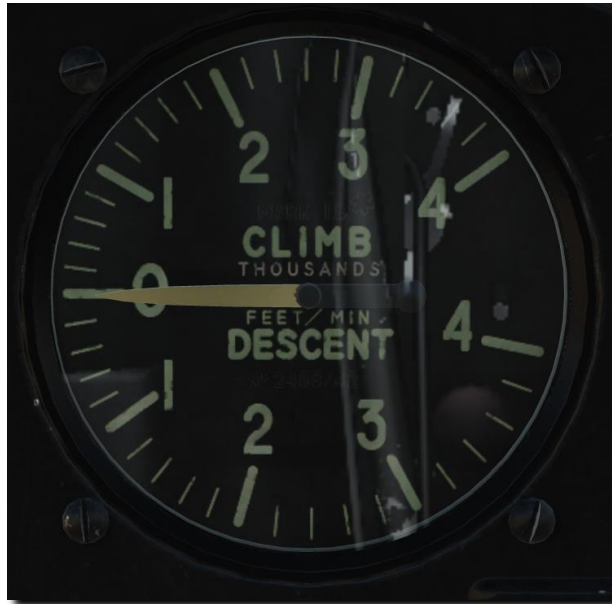
Figure 42: Vertical speed indicator.
