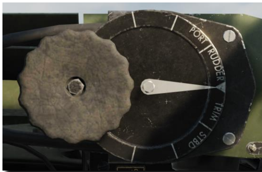
Figure 58: Rudder trim handle and indicator.
