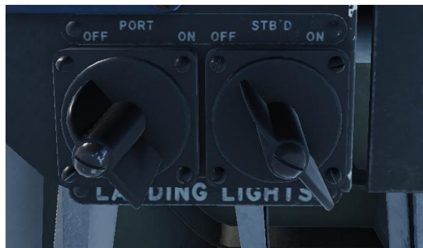
Figure 65: Landing light switches.
