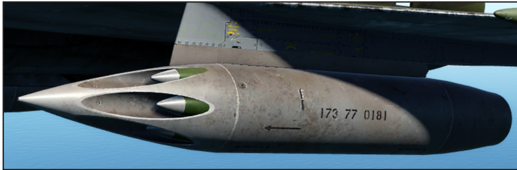
Figure 173. ARAK M/70B rocket pod (HE rockets).
