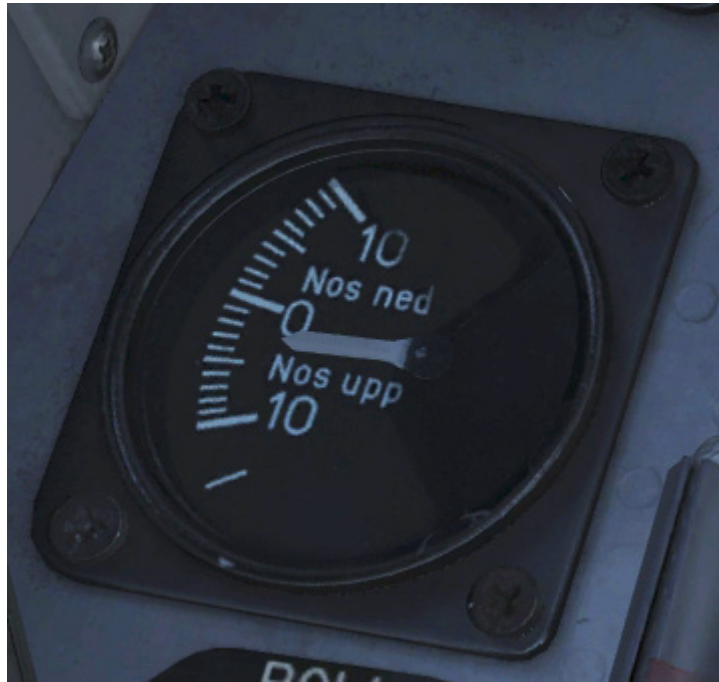
Figure 31. Pitch trim indicator. 3° nose up trim.
