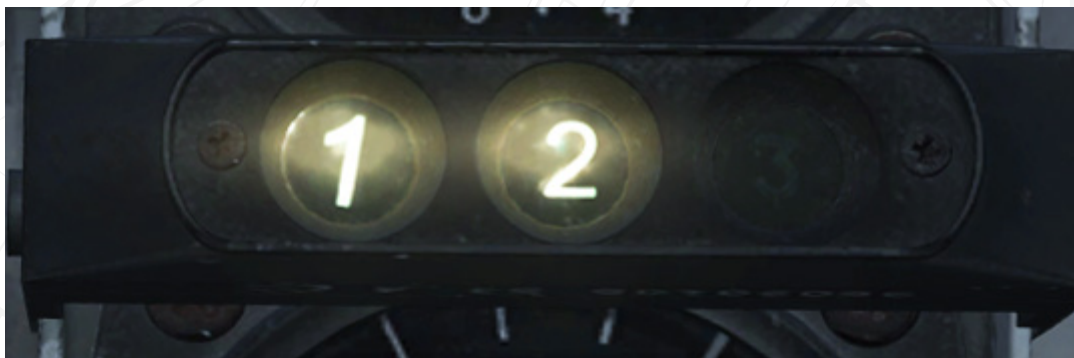
Figure 17. Afterburner indicator. Afterburner Zone 2 selected.
