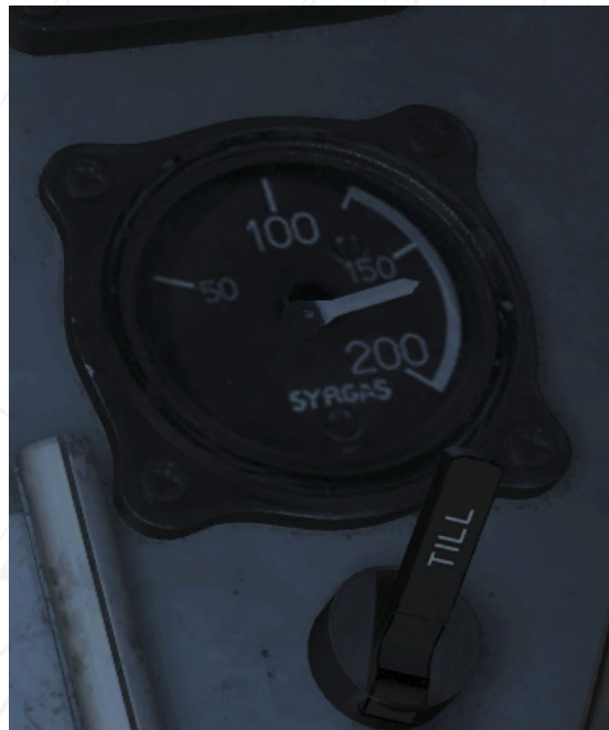
Figure 28. Oxygen pressure indicator. >150 kPa/cm 2 remaining. Oxygen valve in the ON (TILL) position.
