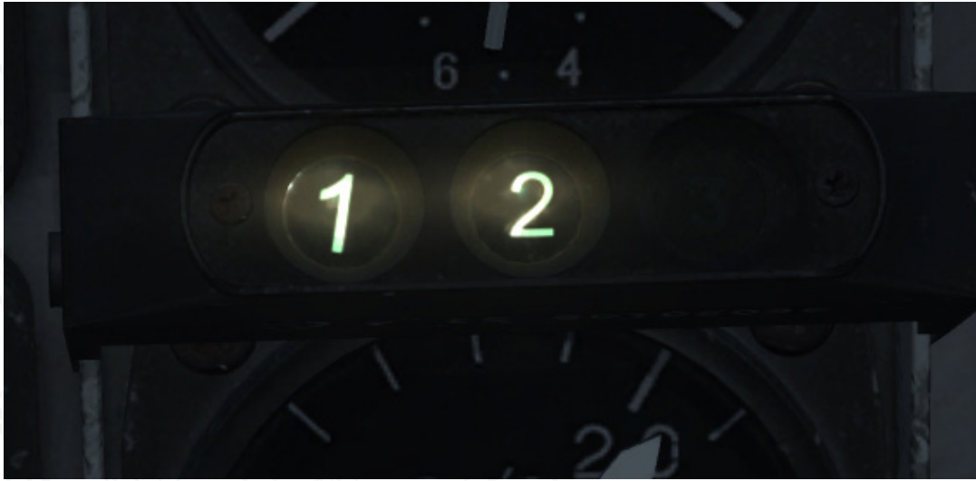
Figure 42. Afterburner zone indicator. Zone 2 selected.
