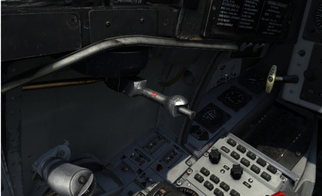
Figure 167. Canopy control lever. In position neutral.
