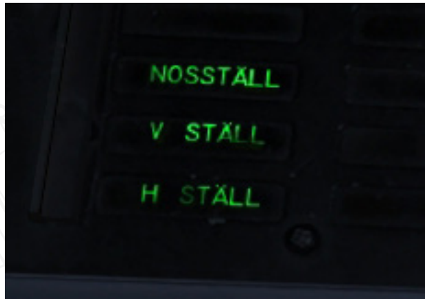
Figure 58. Landing gear indicator on left warning / indicator panel.
