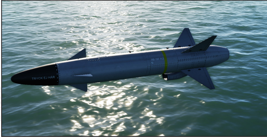
Figure 178. RB-15 Anti-ship missile.
