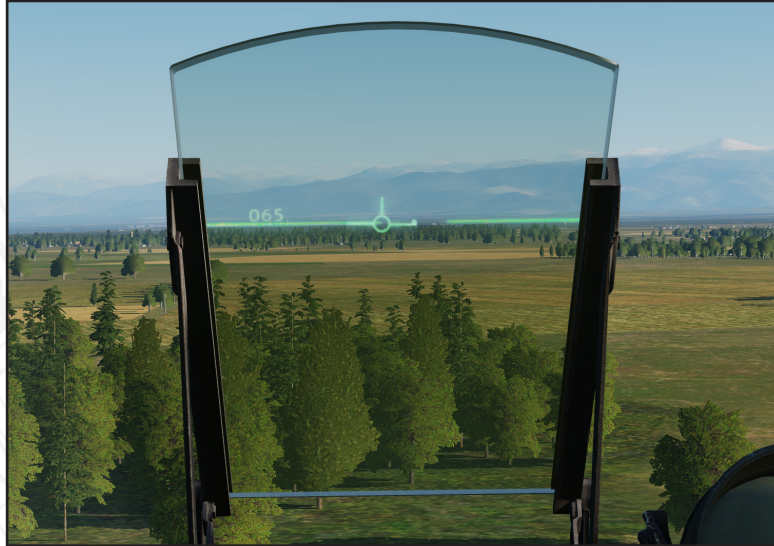
Figure 79. HUD in LOW NAV mode.
