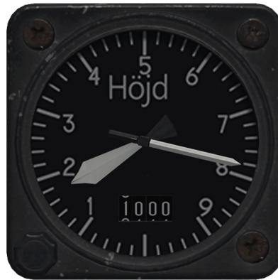
Figure 19. Backup Altimeter. 1780 metres. Pressure set to 1000 hPa.
