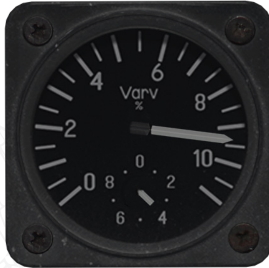
Figure 14. RPM indicator. 94% RPM.
