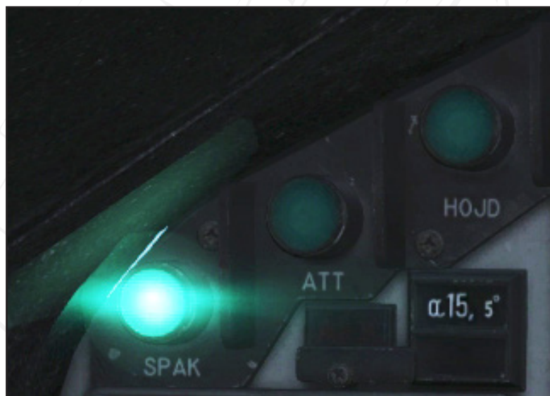
Figure 61. Autopilot mode selector buttons. SPAK mode on.
