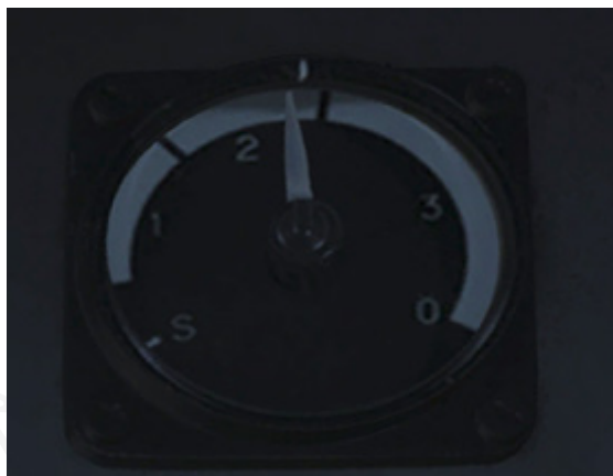
Figure 18. Engine nozzle indicator. Zone 2 afterburner open.
