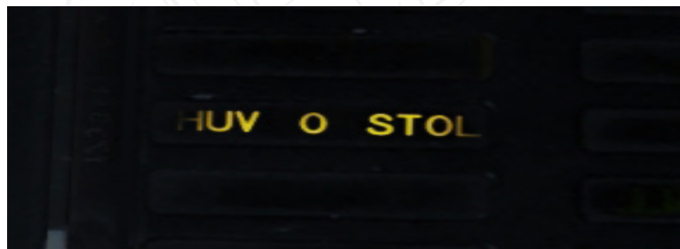
Figure 168. Canopy and ejection seat warning (HUV o STOL)
