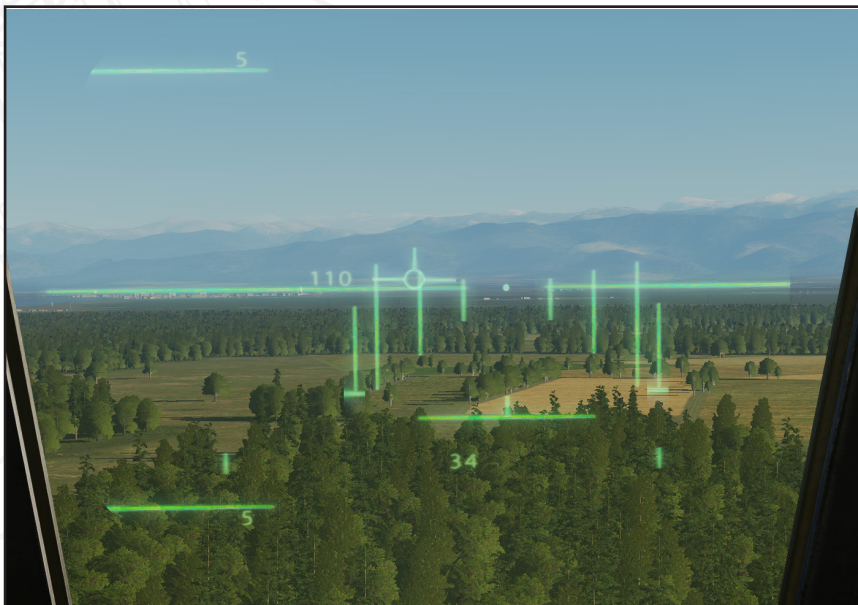
Figure 68. HUD in normal navigation mode.
