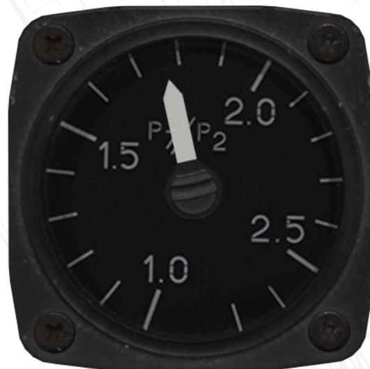
Figure 15. EPR indicator. EPR 1.78.
