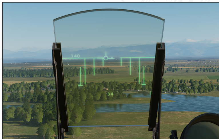
Figure 75. Pole-track with reference bar. Commanded altitude at 140 meters
