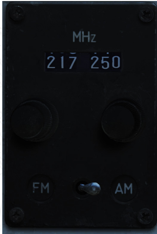
Figure 158. Frequency selector (UHF 217.250 MHz)
