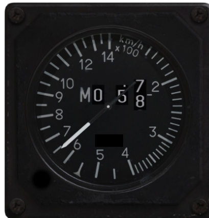
Figure 9. Main Airspeed Indicator. 650 km/h indicated air speed, Mach 0.58
