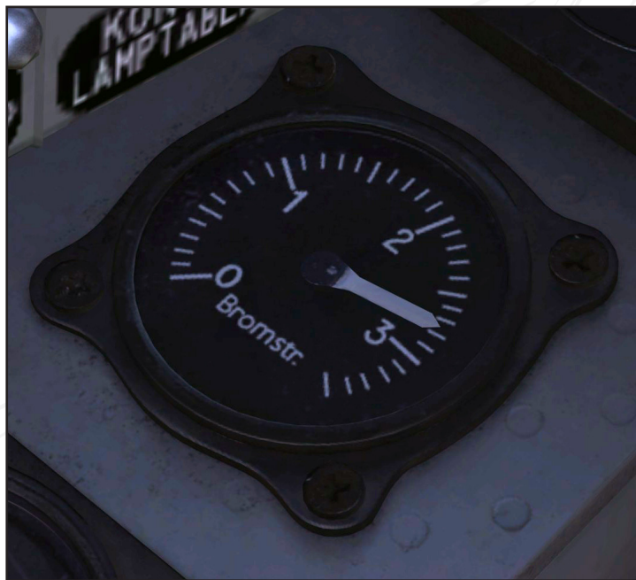
Figure 59. Brake pressure indicator.
