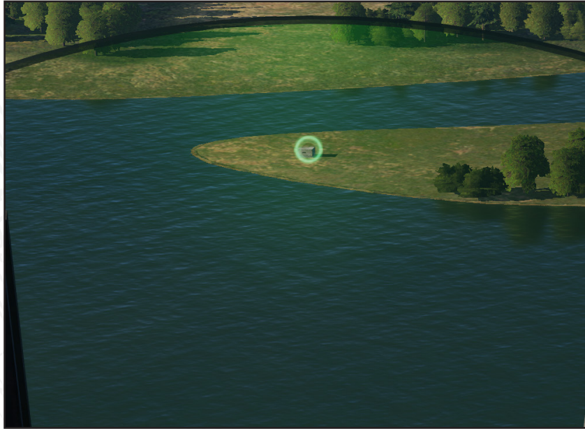
Figure 192. Backup sight symbology (in this case for rockets).
