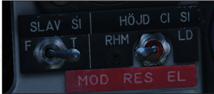
Figure 121. Altitude source selector (right)
