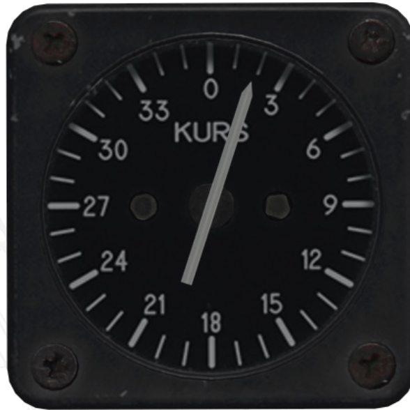
Figure 21. Backup Compass. Indicating 020° Magnetic.
