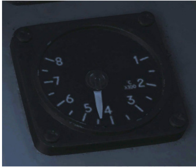
Figure 16. EGT indicator. Approximately. 440° C
