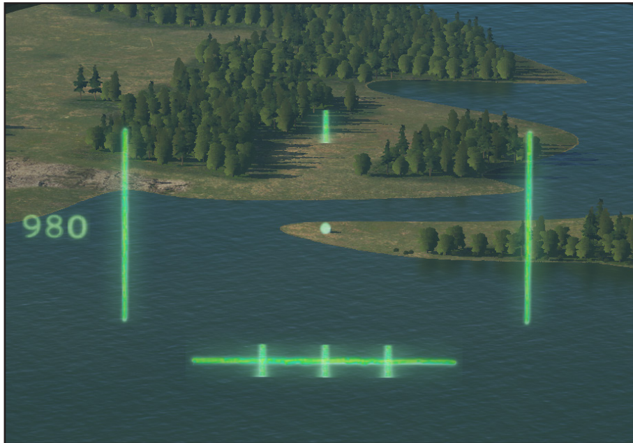
Figure 190. HUD in A/G rockets mode.
