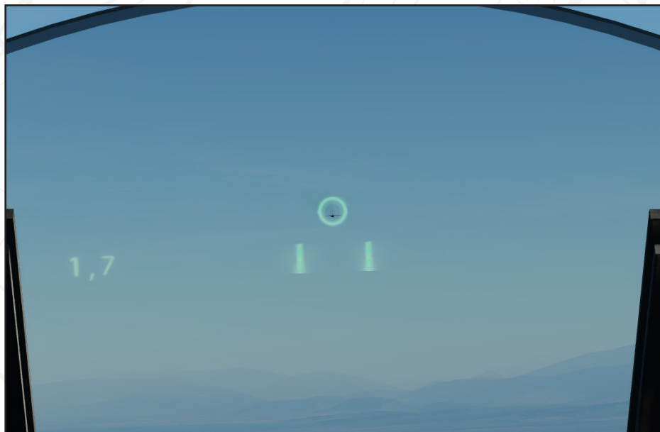
Figure 191. HUD symbology for IR missiles without radar lock with an uncaged seeker.
