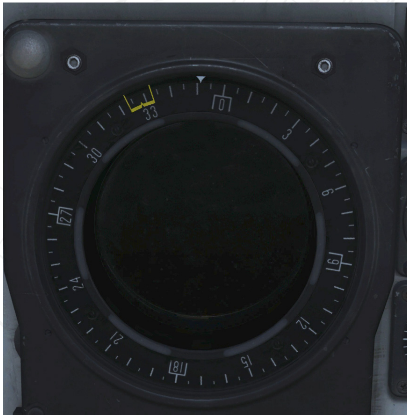
Figure 13. Central indicator with Course ring. Current heading 351. Commanded heading 329.
