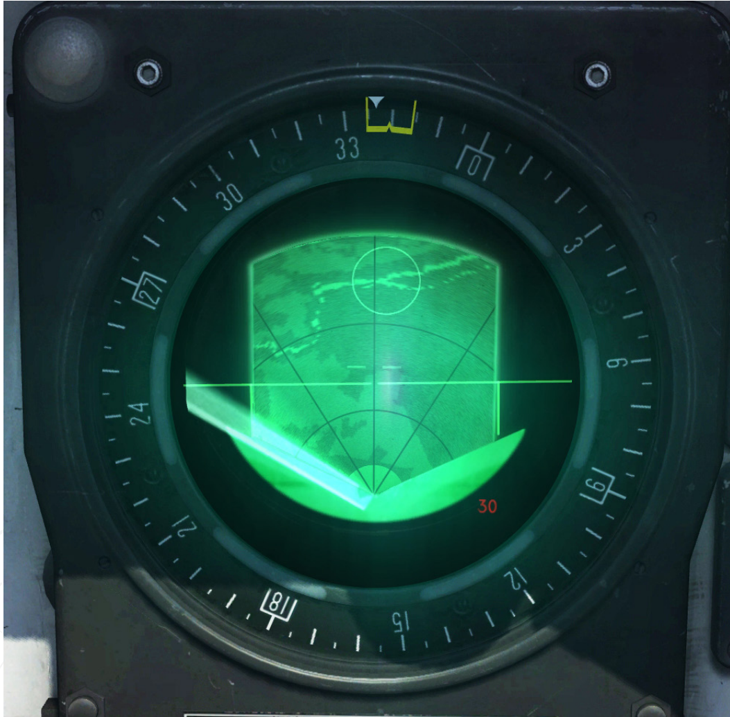
Figure 102. Radar in PPI, 30 km scan zone. Current heading 337, commanded heading 340. Waypoint on an island in the river approx. 27 km away.
