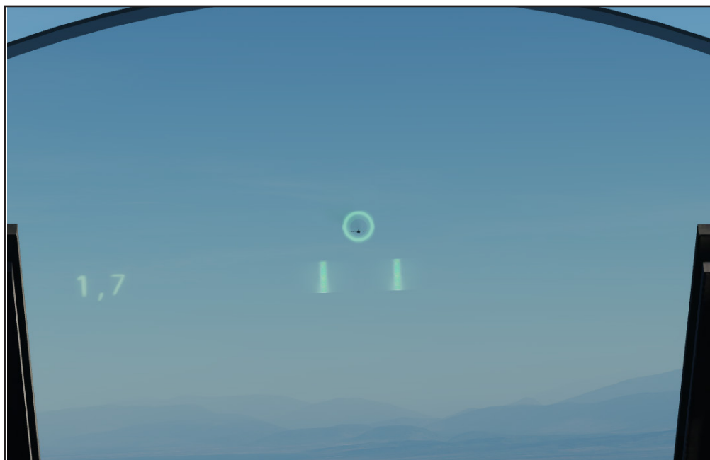
Figure 234. Sidewinder HUD symbology.. Missile uncaged.
