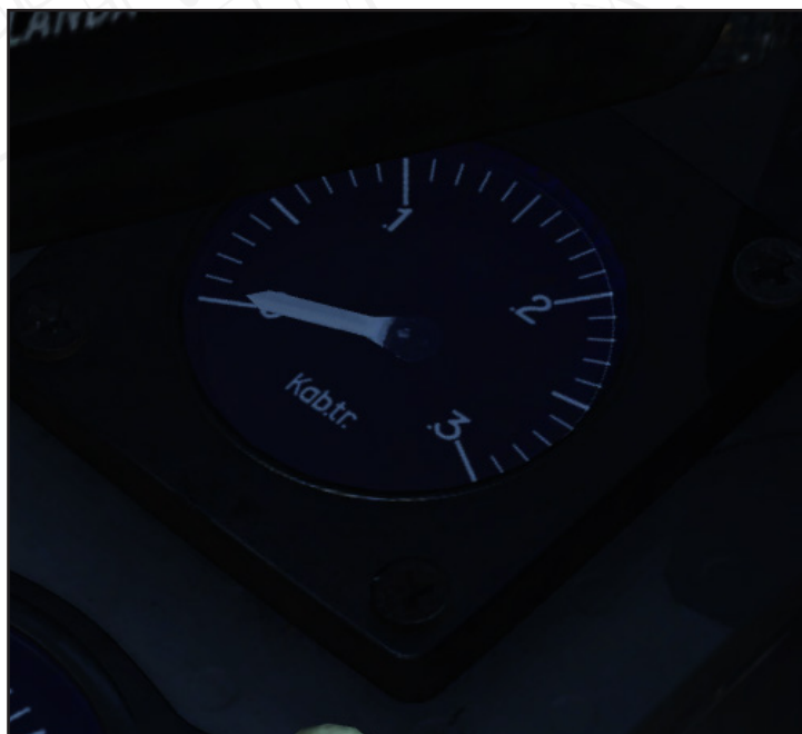
Figure 30. Cabin pressure indicator.
