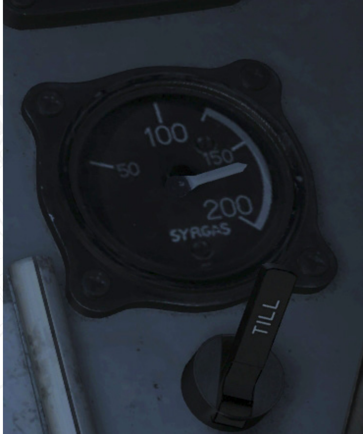
Figure 171. Oxygen pressure indicator (kp/cm 2 ) and oxygen valve ON (TILL)
