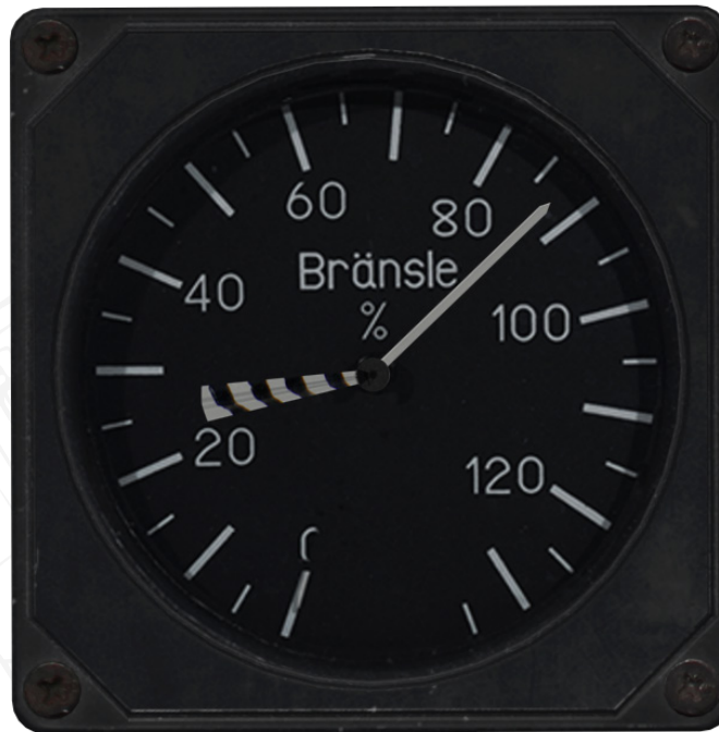
Figure 127. Fuel indicator. 87% fuel remaining. Striped “tie” indicating approx. 30% required to complete flight plan with fuel reserve included.
