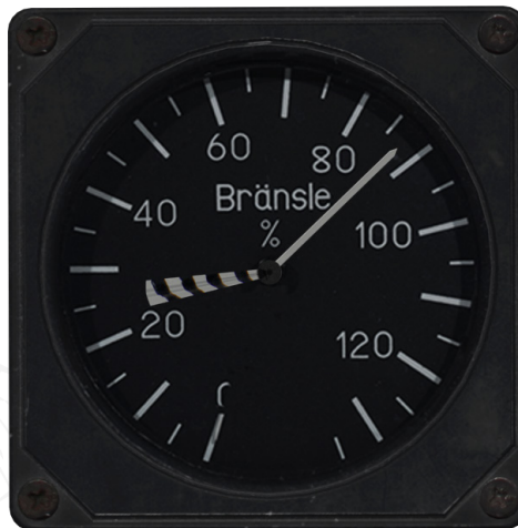
Figure 25. Fuel indicator. 87% fuel remaining. Approx. 30% fuel required to complete flight plan with planned fuel reserve added.
