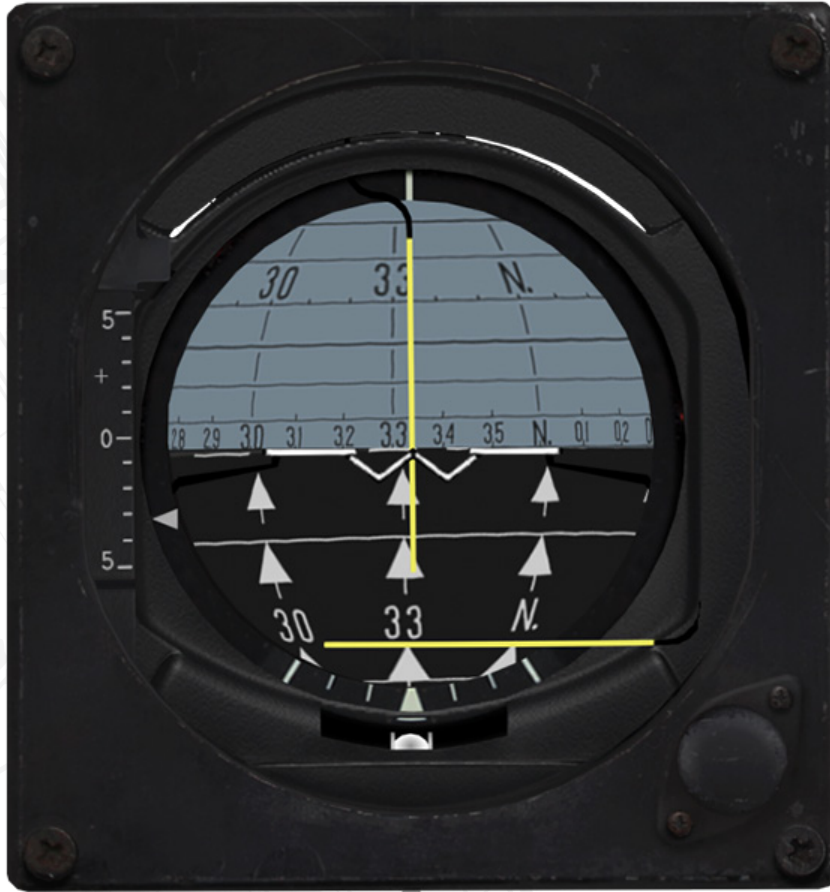
Figure 11. Main Attitude Director Indicator. Straight and level flight, -3 metres per second vertical speed, heading 333, commanded heading 330
