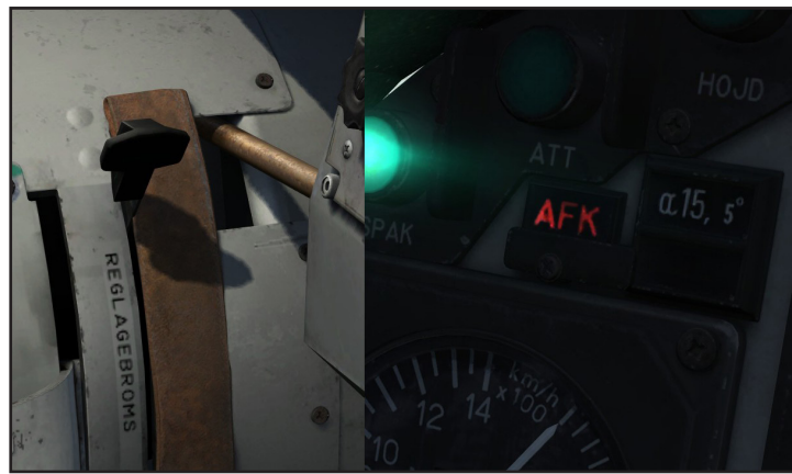
Figure 49. AFK lever and indicator.
