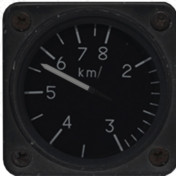
Figure 22. Backup airspeed indicator. 560 km/h indicated airspeed.
