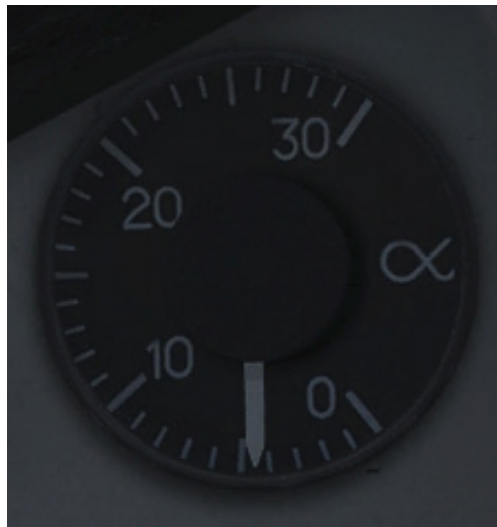
Figure 12. Angle of attack indicator. Indicating 4.5° AoA ( \alpha ).
