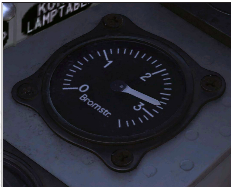
Figure 29. Brake pressure indicator.
