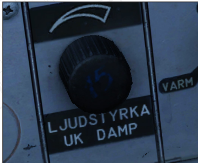
Figure 94. RWR (Master volume) control
