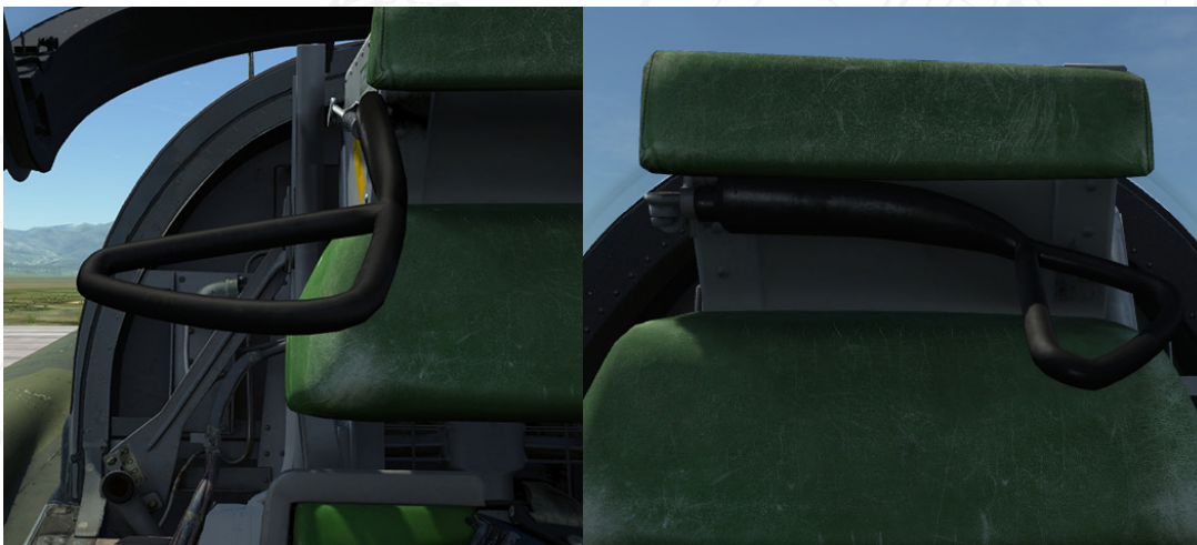
Figure 170. Ejection seat arming lever. Left SAFE, Right (stowed) UNSAFE.
