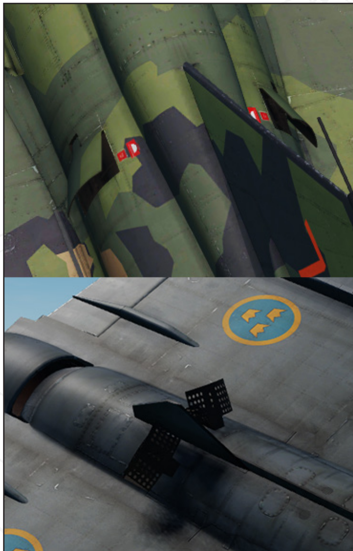
Figure 54. Airbrake system (Upper and lower).
