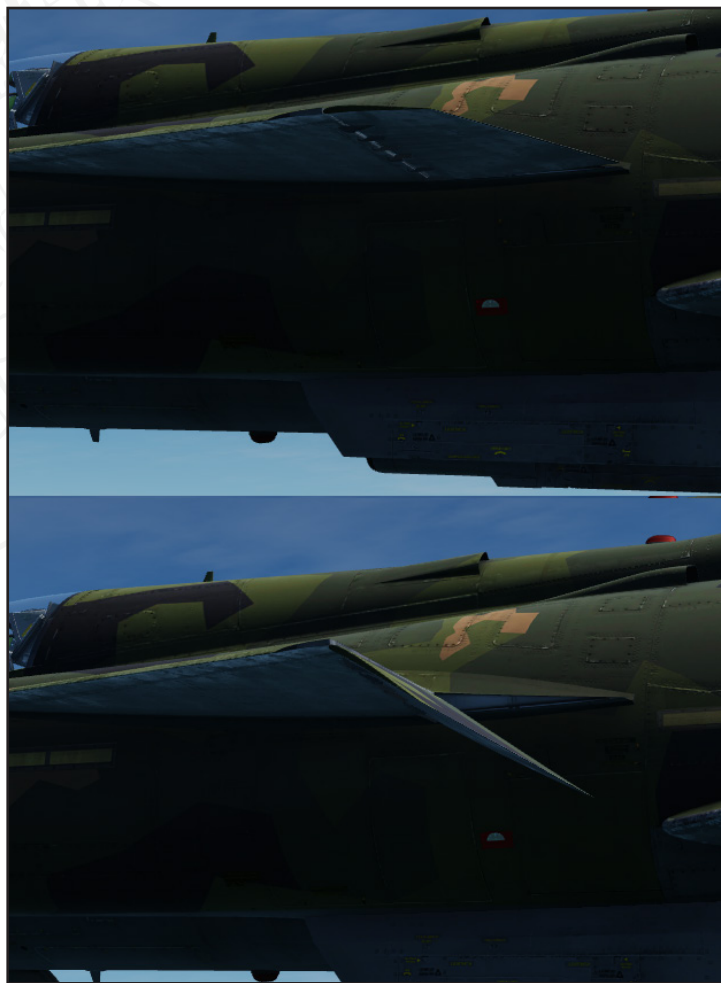
Figure 55. Flaps (raised and lowered positions).
