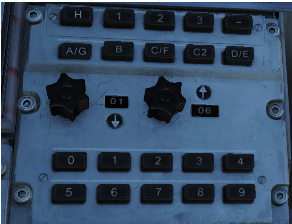
Figure 157. FR 22 radio selector panel Channel A on Base 06 selected.
