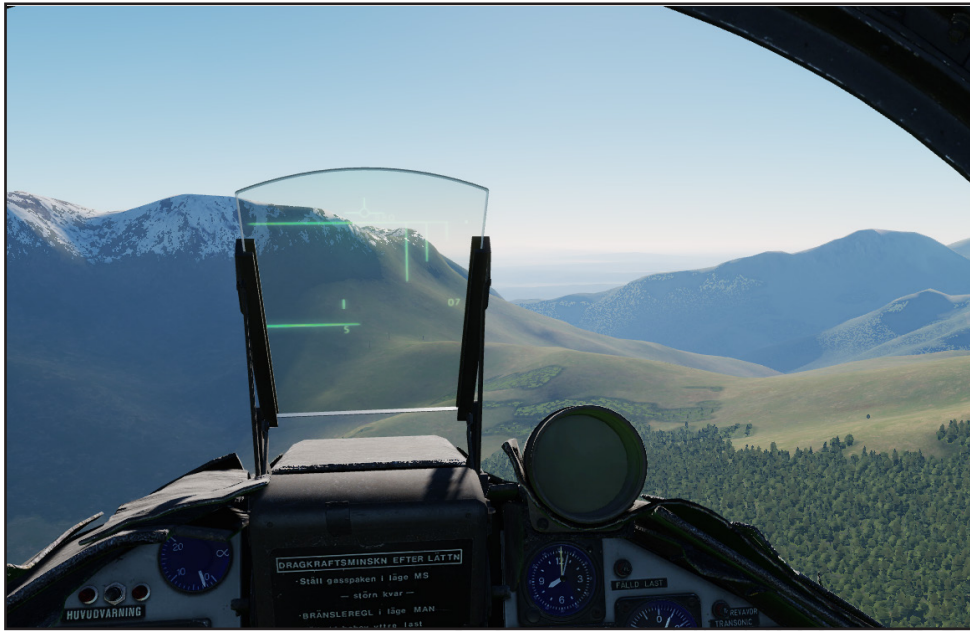
Figure 89. Terrain avoidance mode
