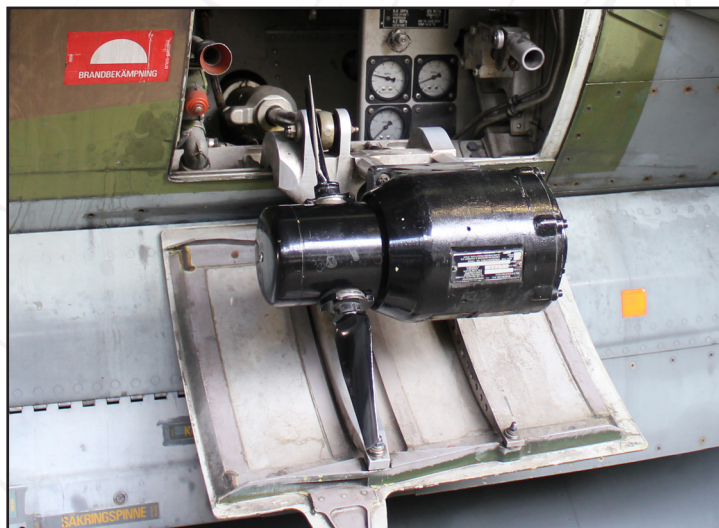
Figure 161. Ram air turbine.
