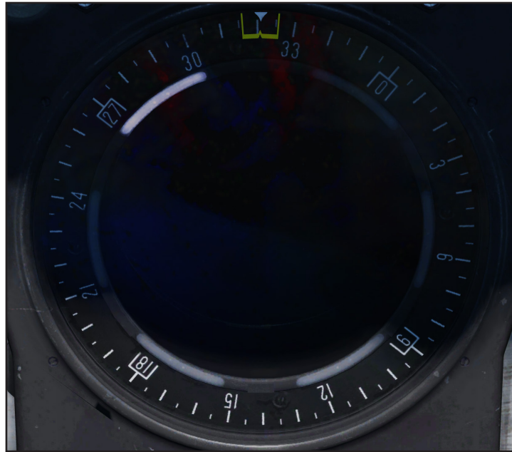
Figure 92. RWR display. Receiving radar signal from 11 o'clock or between 260° - 320° bearing
