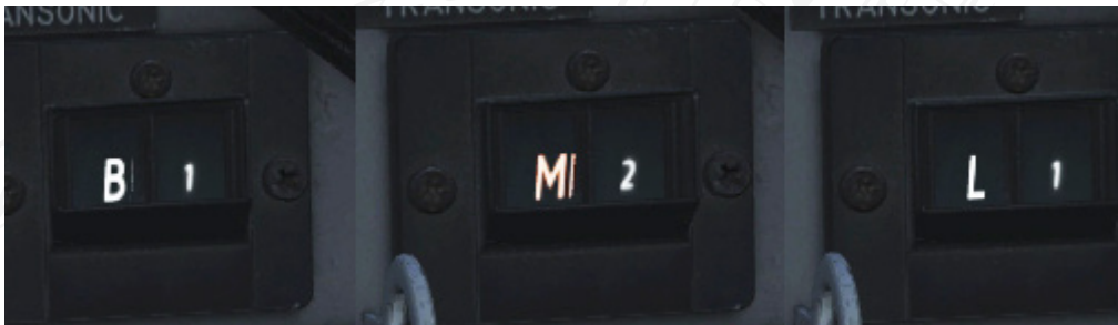
Figure 24. Destination indicator. Left indicating waypoint 1 (B1). Centre indicating target waypoint 2 (M2). Right indicating the primary landing base (L1).
