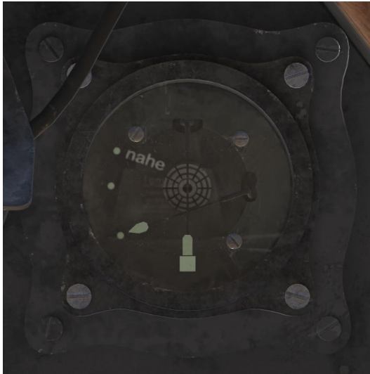
Figure 34: AFN-2 homing indicator
