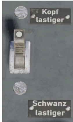
Figure 66: Horizontal stabilizer trim switch
