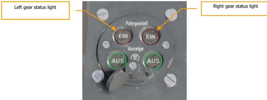
Figure 64: Landing gear indicator
