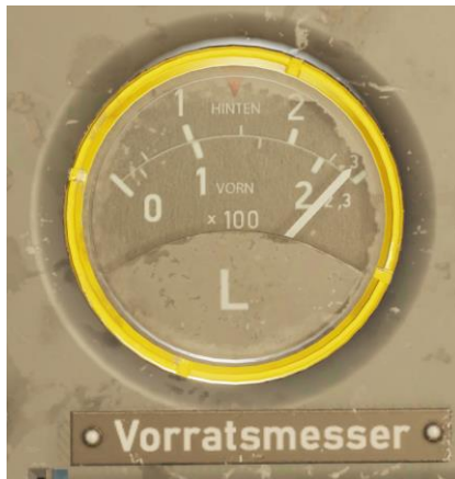
Figure 52: Fuel remaining gauge
