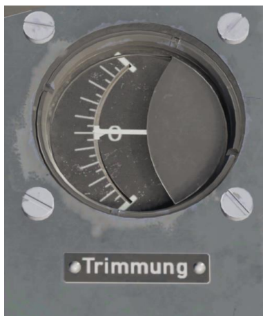
Figure 67: Horizontal stabilizer trim indicator
