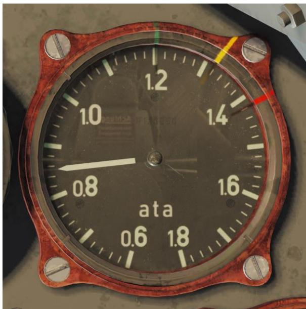
Figure 40: Supercharger pressure gauge
