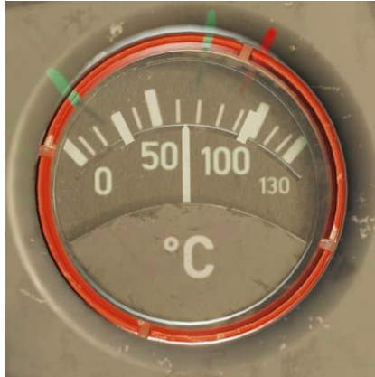
Figure 51: Oil temperature gauge
